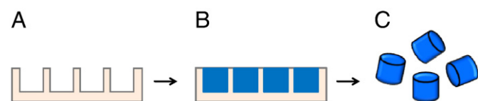
Fig. 1. Schematic diagram showing the fabrication of homogeneous drug-PLGA microparticles using the hydrogel template method. (A) A hydrogel template with wells is formed from the silicon wafer master template. (B) The wells in the hydrogel template are filled with drug-PLGA in organic solvent and then dried. (C) The drug-PLGA particles are obtained by simply dissolving the hydrogel template in aqueous solution.
